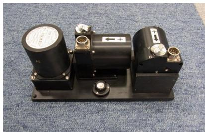
Photo 4 : Servo velocity detectors for microtremor measurement and so on
